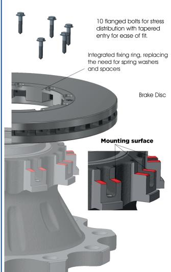
The Fras-Le design is mounted on a different section of the hub and is a larger surface area. A greater surface area has much less wear potential.
