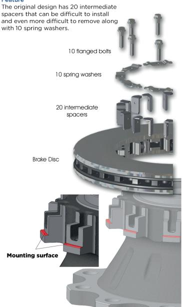
The original design is mounted on a small surface area and is prone to excessive wear. Excessive wear to this area can cause the disc to become loose.
