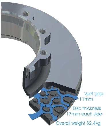
This multi-directional design increases airflow for greater cooling properties. The increased thickness of the braking surface also reduces the rik of thermal cracking.
